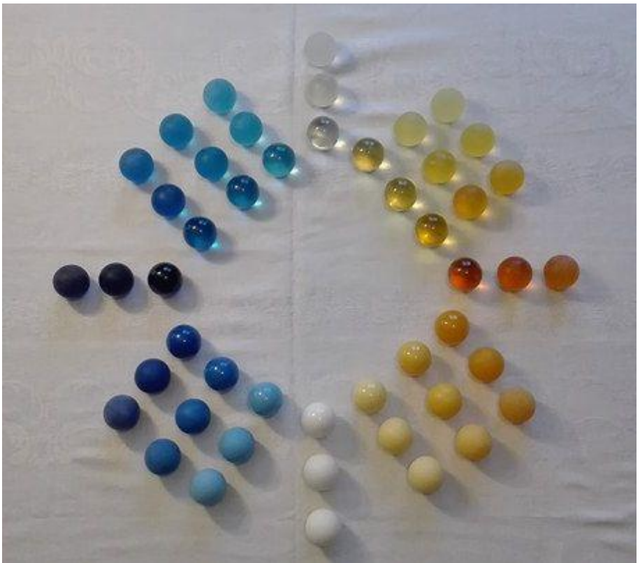
Figure 1: Image of the spheres from transparent to color to white and the three levels of coarseness.
