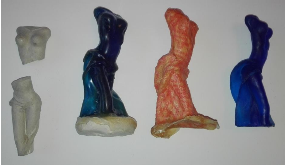
Figure 8: From left to right; Original in clay, broken as per mold creation procedure; one of the liquid latex mold creation; Mold created with liquid latex and reinforced with fabric to avoid deformation; resin object after molding. Three of those objects were created and derived in three coarseness, then served as primaries for the silicon molds.
