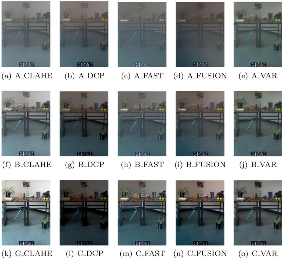
**Fig. 3** The foggy images of scene 1 processed by the selected dehazing methods at fog levels A, B and C
