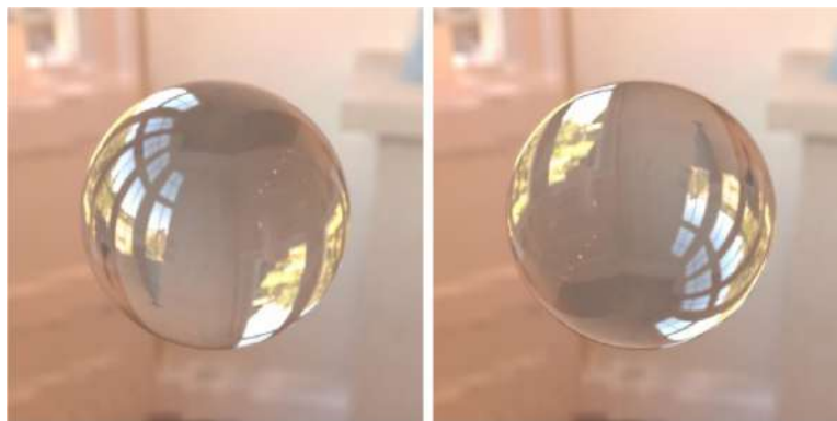
Figure 9. The transmission image in the left photograph is upside-down, which indicates that it is the result of the refraction through a convex lens. If we simply rotate the sphere upside-down, then the transmission image will look more like an opaque mirror reflection. This was first demonstrated by Kim and Marlow (2016) .
