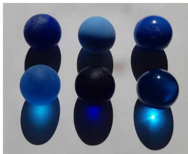
Figure 17. Although the object body might look fully opaque (e.g., the middle object in the bottom row), the external caustics provide rich information about the subsurface light transport properties of a material. The figure is reproduced from Gigilashvili et al. (2019a) . The animated version can be seen in Supplementary Material 2.
