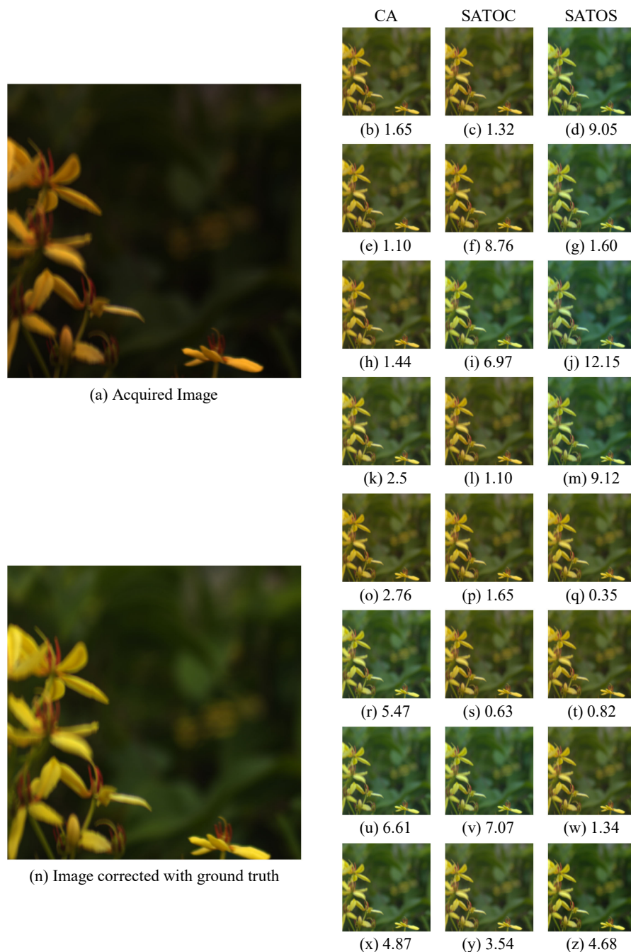
Fig. 10. Images on the right are obtained by applying the illuminant estimation for the color correction. We report the recovery error in degrees in the caption below the images. The images are arranged in three columns, each representing a different model (CA, SATOC, SATOS), and eight rows, each representing a different patch size ranging from 4 to 512.
