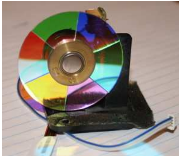
Figure A.12: A color wheel with 6 primaries. Note that the size and the arrangement of each color is not the same to avoid some color breaking effect. From http://www.jangro.com/images/samsung-dlp/samsung-color-wheel.jpg .
