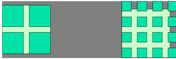
Figure A.3: Illustration of the variation of luminance with the resolution. The surface covered by the material used to fix the liquid crystal films more and more of the panel surface while increasing the resolution.
