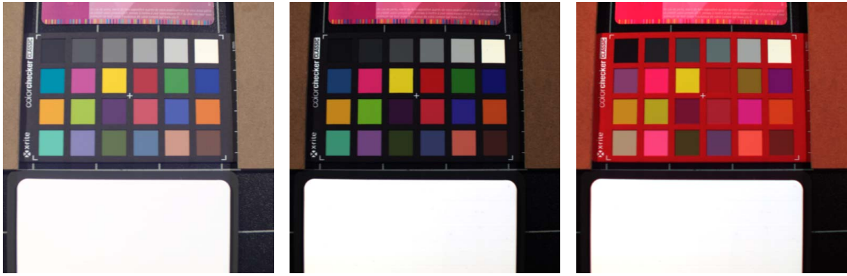
(a) Color reconstruction: with a D65 illuminant and a sRGB ICC profile, to be visualized on a sRGB monitor (b) Spectral reconstruction: 650 nm assigned to the Red channel, 550 nm to the Green and 450 nm to the Blue channel (c) Spectral reconstruction: 850 nm (IR) assigned to the Red channel, 550 nm to the Green and 450 nm to the Blue channel
