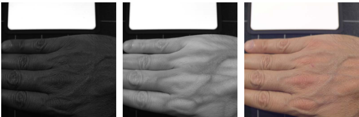
(a) Spectral reconstruction: 450 nm assigned to the Red, Green and Blue channels (b) Spectral reconstruction: 850 nm (IR) assigned to the Red, Green and Blue channels (c) Color reconstruction: with a D65 illuminant and a sRGB ICC profile
