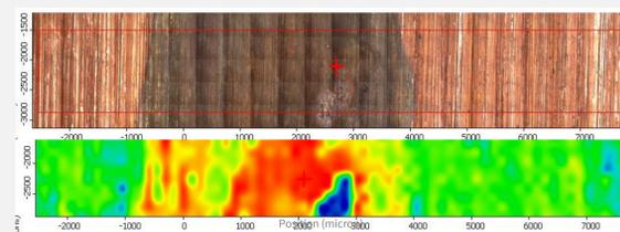
µFTIR chemical image of copper palmitate on a LO-coated copper coupon after 2 months accelerated ageing at RT and 75% RH (NaCl saturated solution in water)
