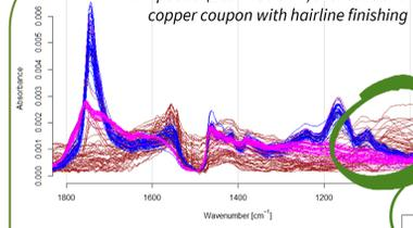
The FTIR spectra collected in RA mode are affected by the hairline finishing, resulting in low reproducibility when no coating is applied (dark red line). This is well represented by the Principal Component Analysis (PCA).
