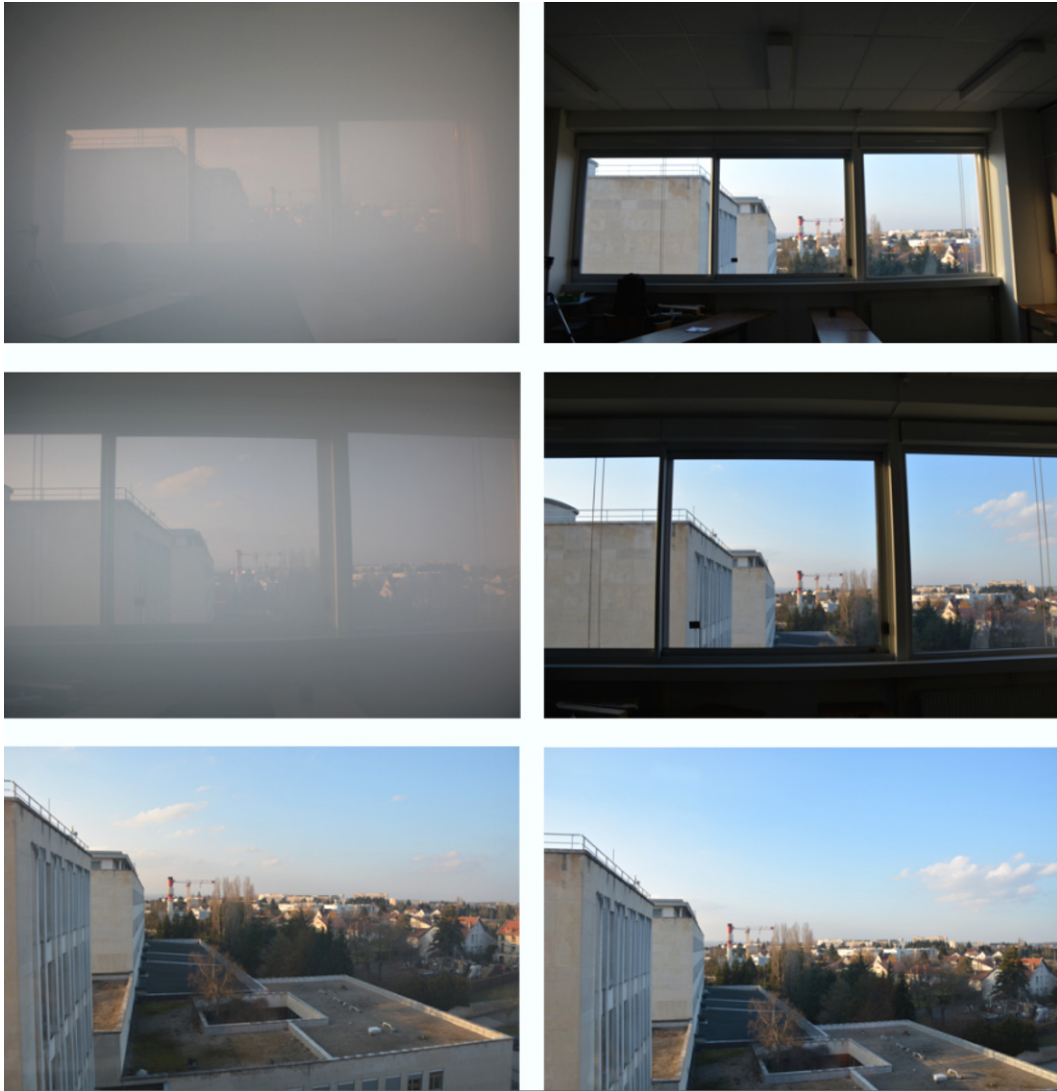
Figure 7. Dynamic scene. The left column shows images with fog taken at 5.6 m (level 1), 3.5 m (level 4) and 0 m (level 9) from the window, respectively. The right column shows the fog-free images taken at the same distances.
