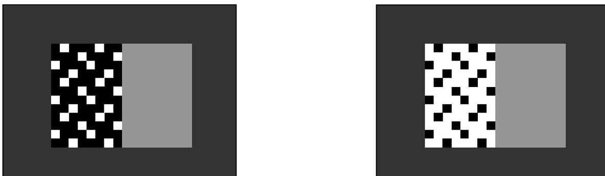
***Adding two new luminances ( 25% and 75% ) to determine the camera response curve***
